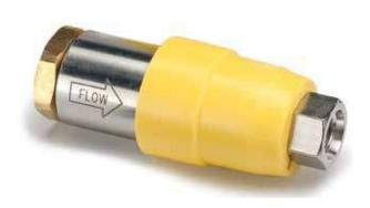
Parker's NGVBCN2-P50 fill line breakaway provides an important safety feature for CNG dispensing systems. It is certified to ANSI/NGV4.4/CSA12.54 standards for breakaway devices used on natural gas dispensing hoses and systems. It allows the hose to safely disconnect, preventing damage to the dispenser in the event of a "drive off" and sealing the CNG in the fill line to effectively prevent leakage or hose whip.
