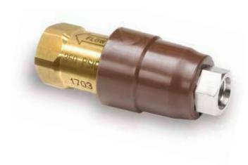
Parker's vent line breakaway provides an important safety feature for CNG dispensing systems. It allows the vent line hose to safely disconnect, preventing damage to the dispenser in the event of a "drive off" and allows any CNG remaining in the vent line to bleed off safely.
